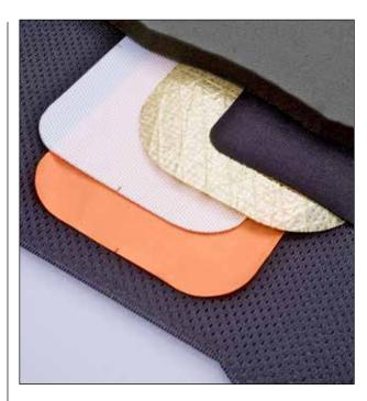
The Elektron Laser ZP cut most synthetic fabrics quickly, accurately and with minimum edge discolouration.
